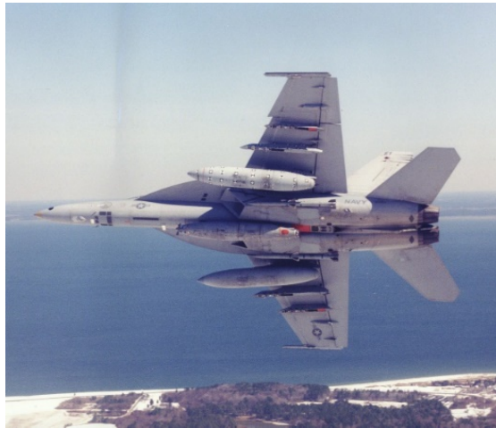
Figure 15: F-18E/F Pylon Toe.
